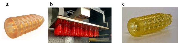
Figure 1: a) CAD rendered image of a screw design, b) Build plate immediately after 3D printing step, c) Fully cured 4Degra® interference screw.
